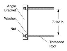
that the posts have to fit inside the mounting clamps (assuming you wish to use the hardware provided by Electro-Mech). The standard clamps form a "pocket" that is 7-1/2 inches square. So, if you try to use a 10-inch diameter pipe, our clamps will not work.
